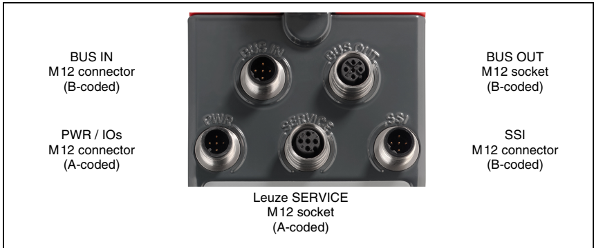
Figure 7.1: Connections of the AMS 304 i
